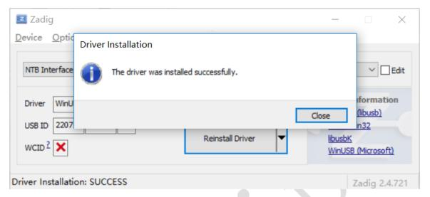
■ After installation, if the TB-RK1808 AI Compute Stick in the Windows Device Manager does not have an exclamation point, and as shown below, the installation is successful.
